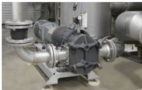
ONIXline pump for conveying C starch
