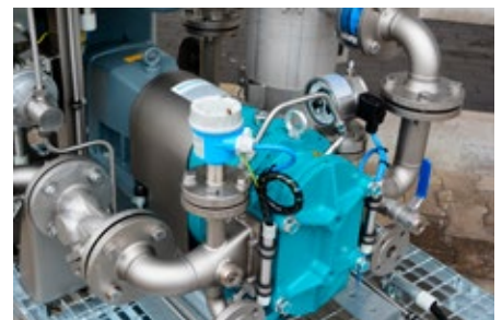
Pressure measurement by means of pressure transmitter
