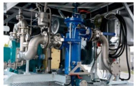
Filter system with differential pressure measurement
