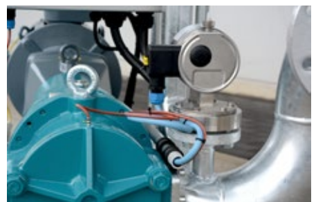
Dry run protection by temperature measurement in the pump chamber
