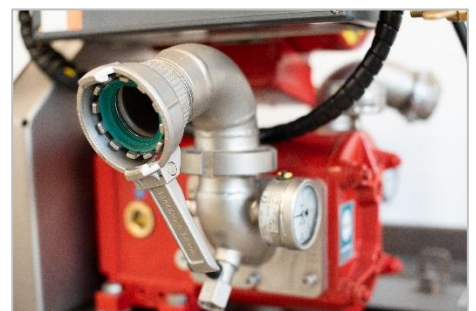
Tanker truck coupling (TW) DN 50 at suction and pressure side
