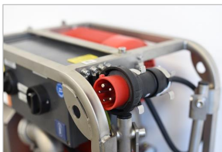
Power supply via an explosion-proof connector
